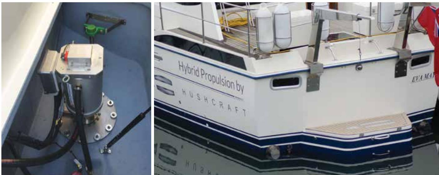
*The 15kW electric motor on the Princess was mounted in a customized bathing platform 'pod'*
