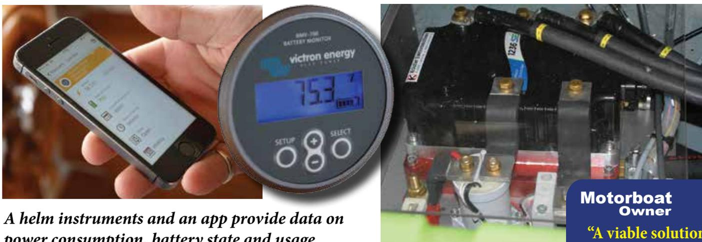
*A helm instruments and an app provide data on power consumption, battery state and usage*
