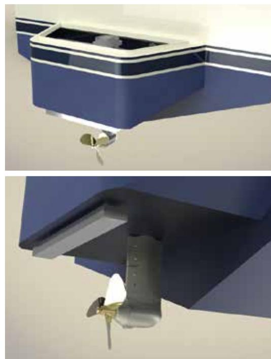
*The drive is connected to the rudders and is steerable up to 45°*
